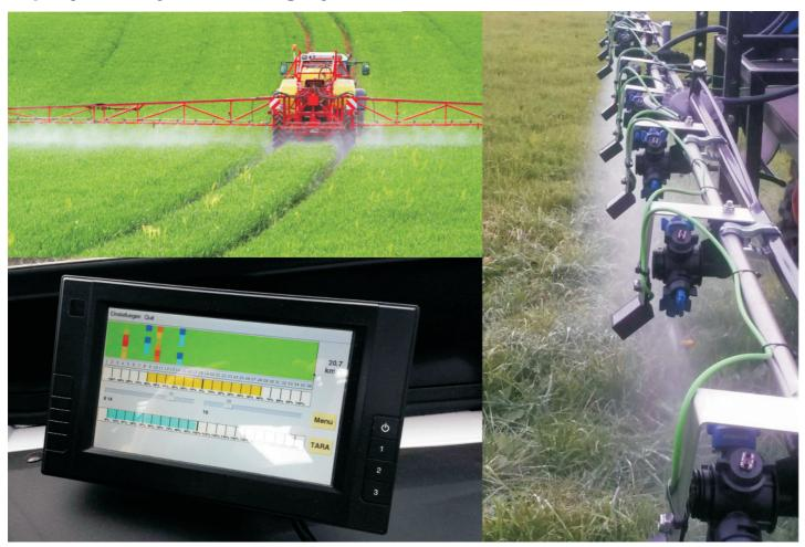
The SprayMon provides for a system monitoring the function and working quality of each nozzle of a sprayer.
