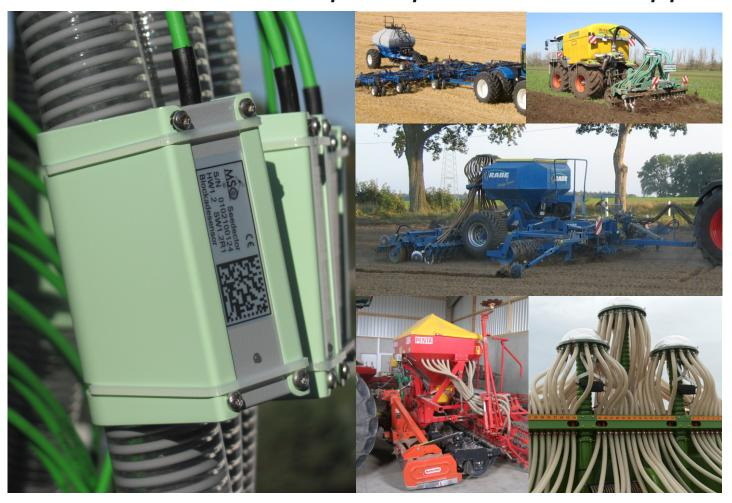
**SeeDector** deploys a microwave doppler technique ("Radar") for detecting mass flow and flow speed of particulate products in hoses / pipes - pneumatically conveyed or free falling.
