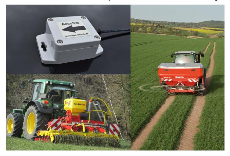
The **AccoSat System** combines the advantages of DGPS-based speed measurement with the high dynamics of a 3D accelerometer. Thus a reliable and fast true ground speed measurement is achieved.
